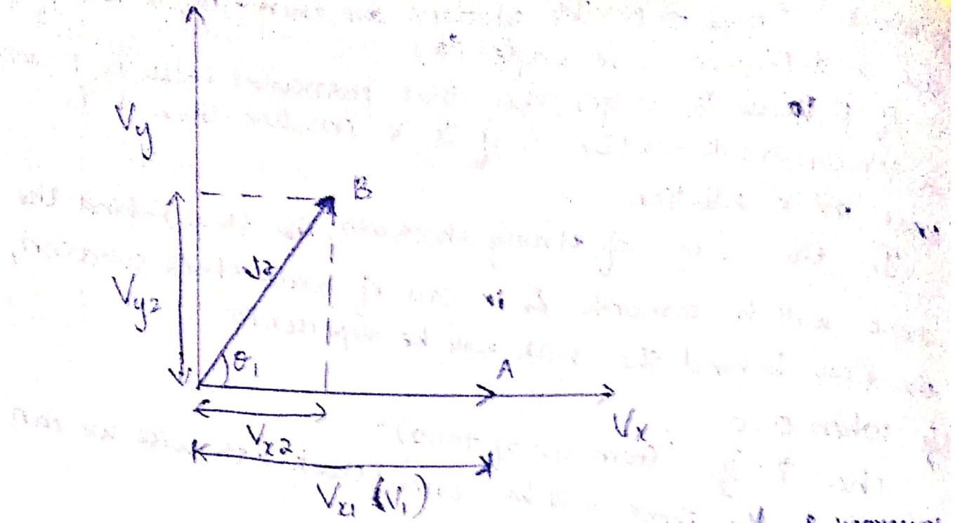
→ Point 'A' represents region 1 in  $xy$  plane and 'B' represents the region 2 i.e., A - flow field ahead of the shock, B - flow field behind the shock.
