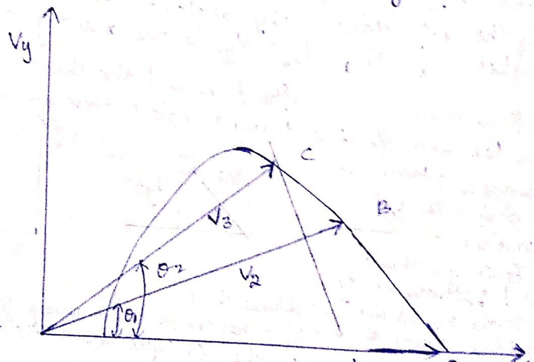
→ The locus of all such points for  $\theta$  values from zero to  $\theta_{\max}$  representing all the possible velocities behind the shock. It is called the shock polar.
