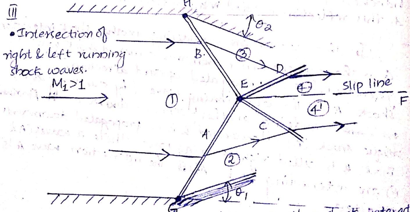
iii In this case we are considering another shock interaction. Here 'G' is the concave corner. From this corner, an oblique shock wave is generated and it is propagated in upward direction. Shock A is the left running concave (by viewing from H). We are considering another concave
